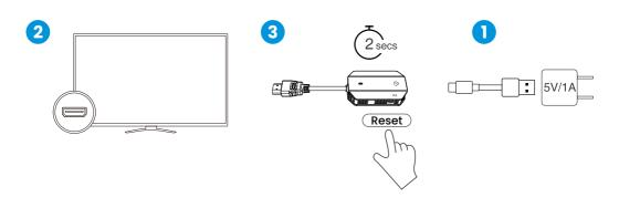
**B.** Press the screen projection/pairing button on the wireless transmitter (TX):
