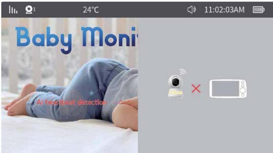
6. **Quad-Split Screen Mode:** This mode is available only when three or four cameras are paired. To activate it, press and hold the camera toggle button in sequence to enter quad-split screen mode.
