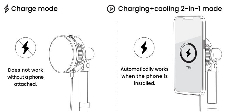
2. When the mode is set to cooling, the radiator automatically begins operation.
