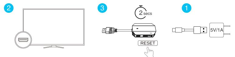
2. Press the Screen Projection/Pairing Button on the Wireless Transmitter (TX):
