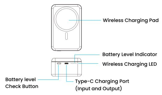
To wirelessly charge an iPhone that supports wireless charging, simply place your iPhone on the product (as shown in the figure). It will automatically attach to the wireless charging pad, and the power bank will detect it.
