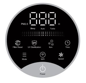
**Power on:** Upon activation, the machine emits a single buzzer sound, the power indicator turns red, and the machine enters standby mode.
