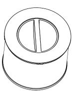
2. Press this button for 3 seconds to reset the replacement reminder. Note: Resetting the reminder does not affect the accumulated operational time.
