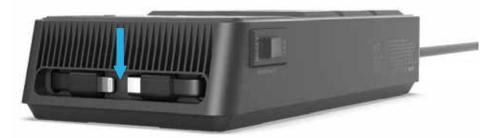
Step 2: After removing the cable joint, gently pull the wire in the vertical direction. When a "click" sound is heard, the cable is fully
