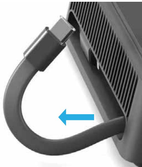
**Step 3:** To retract the cable, gently pull the wire in the vertical direction. When the "click" sound is heard, slowly release it, and the wire will automatically retract.
