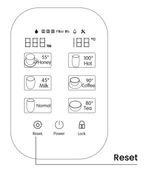
Press and hold "RESET," then touch "RESET" again to select the corresponding filter element. Press and hold "RESET" for 3 seconds to complete the reset process. **Note:** The original filter element must be used for replacement to ensure the safety of drinking water. If any issues occur during the filter replacement process, please contact the professional service agents.
