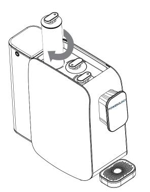
Assemble the new filter element and rotate it clockwise to secure it. Rotate the filter element counterclockwise and lift it out.
