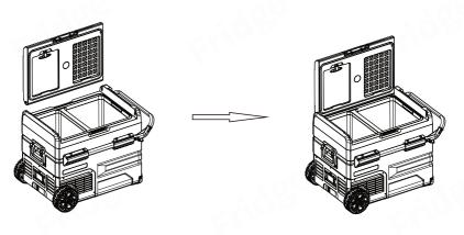
Align the door shaft with the compartment hole and insert it
