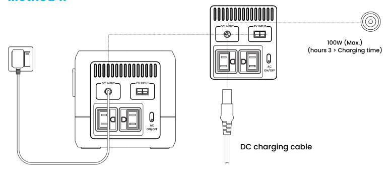
To charge the power generator, insert one end of the supplied adapter cable into the DC port (as indicated in the accompanying image) and connect the other end of the cable to the electrical outlet
