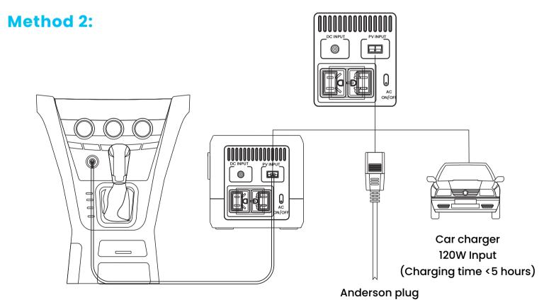
Charge the power generator by connecting the Anderson cable to the cigarette lighter port. Connect the other end of the Anderson cable to the power generator. Important Note: Do not attempt to charge the portable power generator with the car charger while the vehicle's engine is off.
