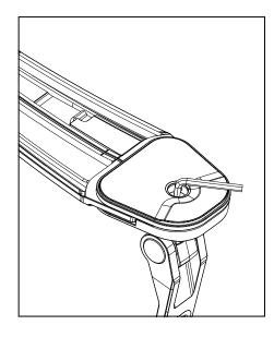
Step 4: Use the large Allen key to modify the tightness of the base.
