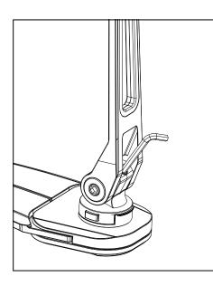
Step 3: Employ the medium Allen key for adjusting the vertical tightness.
