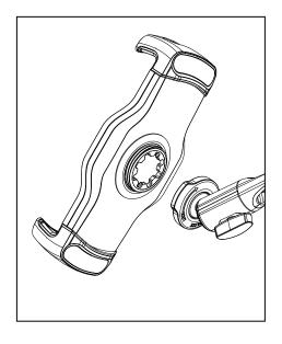
Step 1: Turn in the direction indicated by the arrow to secure the collet in place.
