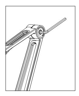
Step 2: Utilize the large Allen key to adjust the vertical tightness.
