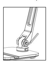
Step 4: Utilize a large Allen wrench to adjust vertical tension.
