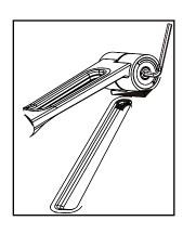
Step 3: Use a large Allen key to fine-tune the vertical tightness for secure positioning.
