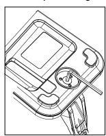
Step 6: Use a large Allen wrench for base tension adjustment.
