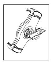
Step 2: Adjust the tightness of the collet's rotation by turning it to the desired resistance level.
