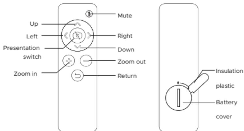
1. There is a insulation plastic with battery, it need to be removed for first use.
